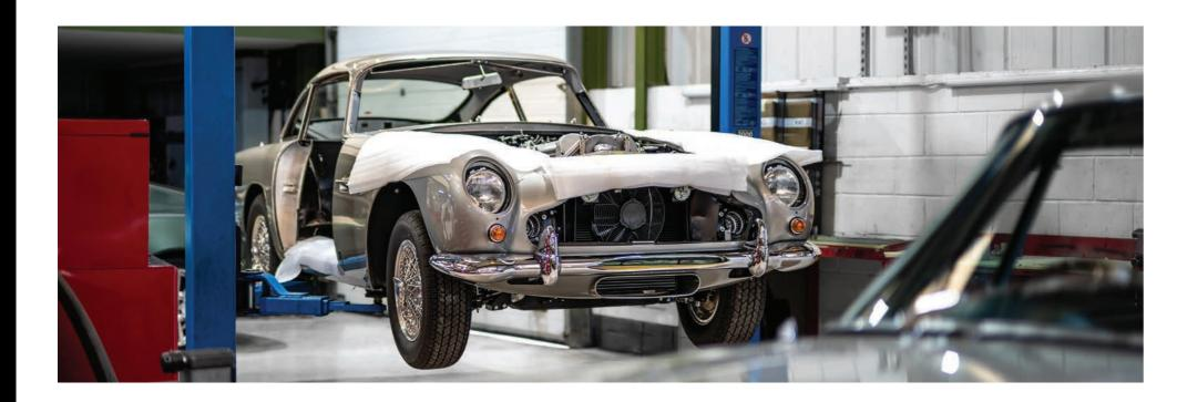
panels to match the original curves and radii of the original body. Once the body and chassis work has been completed the 300+ hour paint process can begin, with countless layers of primer, paint and lacquer applied (hand-blocked between every layer) until a world-class finish is achieved.
